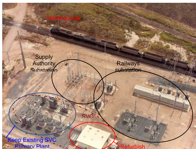
Figure 2 – Railway SVC layout and refurbish decision
